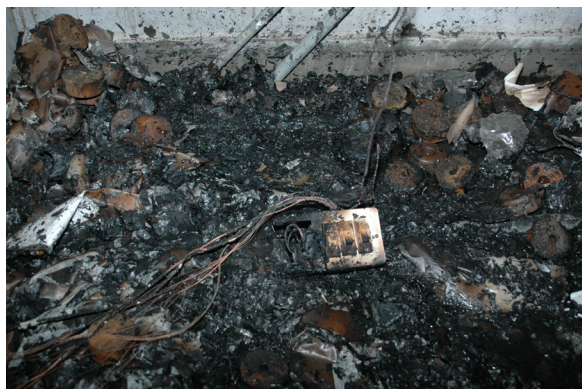
Figure 4: showing the externally mounted wooden extension board at the heat affected corner.
