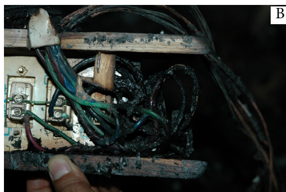
Figure 5: (A): close-up of front side view of the electric circuit board; while in photograph 5(B): Close-up inner side view of the electric circuit board and heat affected insulation is shown.
