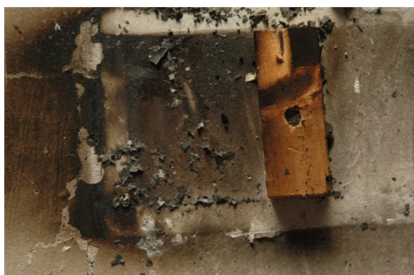
Figure 6: showing metallic globules on the wall where the electric circuit board was mounted.
